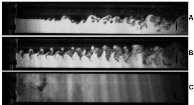
Graceflow fast pipeline mixing technology: (A) unforced mixing in a pipe; (B) mixing under conventional forcing; (C) rapid mixing under our new forcing mechanism. (Image Courtesy: Dr. Hong Jiang)
