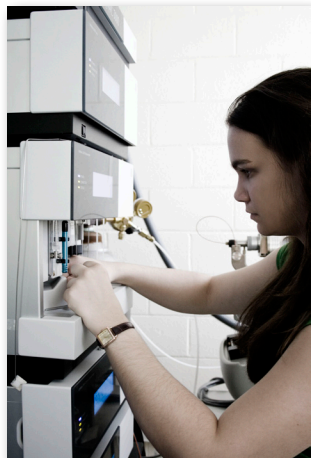
Sarah Spell loads SPE water extract samples onto HPLC triple quadrupole mass spectrometer for trace MRM analysis.
